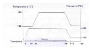
Note: Heat-up rate:3.0-5.0 $^{\circ}$ /min(70-130 $^{\circ}$ )
