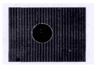
Fig. 7 SP120N (1080prepreg) hole wall quality
